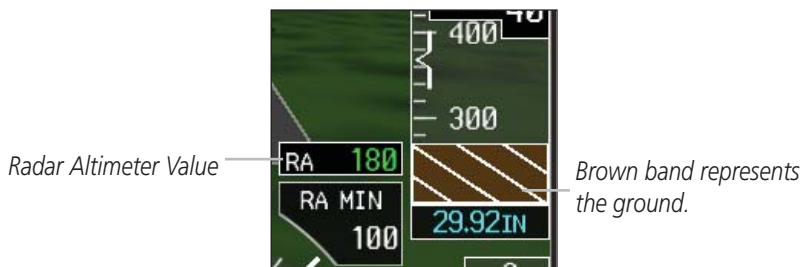
Minimums Annunciations using RAD ALT for Source
